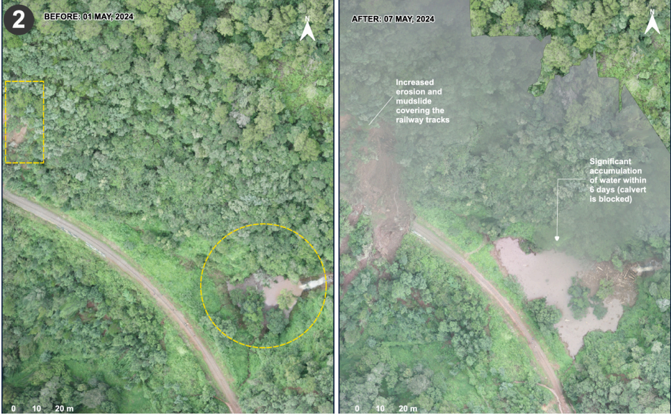
Image 2: A map of the landslide in Mai Mahiu captured by the Wingtra One drone
