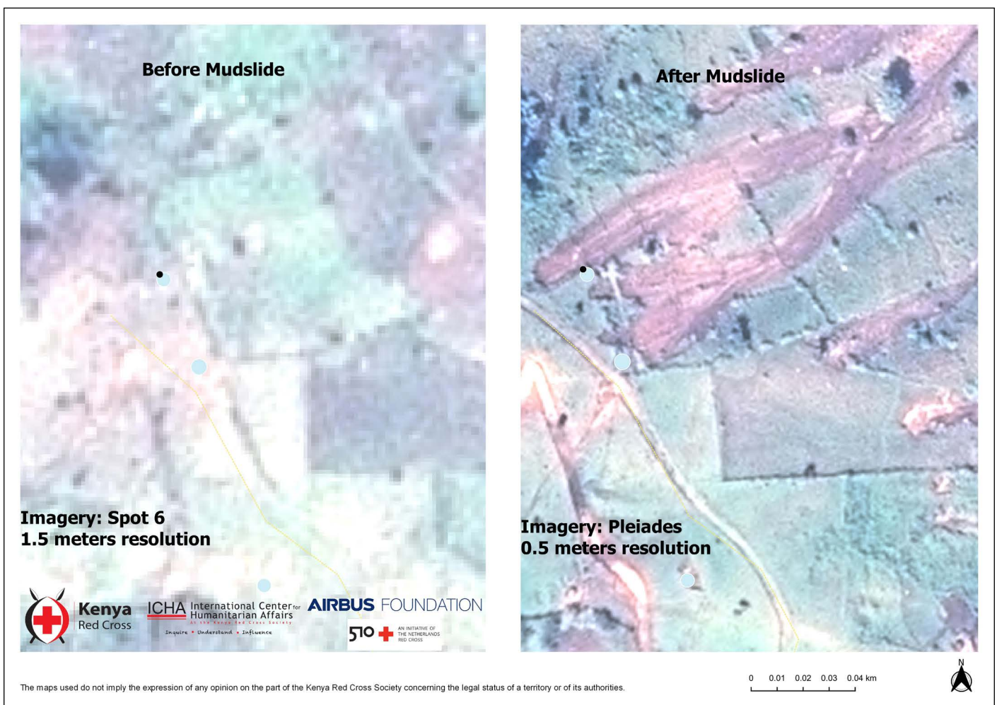
Figure 7: Change detection – visual comparison of spot 6 and Pleiades imageries was done in order to visually interpret landslide scars
